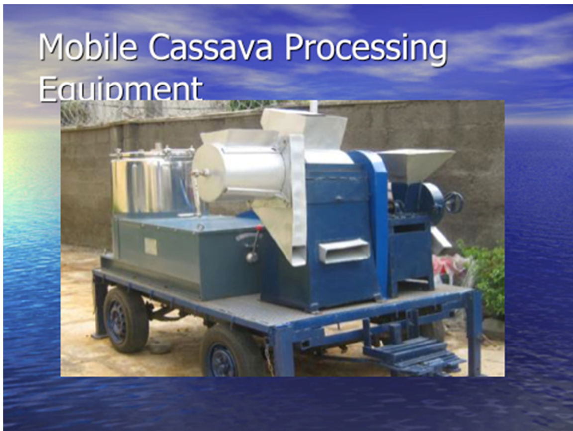
AN EXAMPLE OF A MULTIPURPOSE EQUIPMENT FOR THE CASSAVA COTTAGE INDUSTRY
